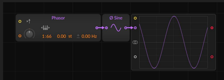
Generating sine wave using phase generator
